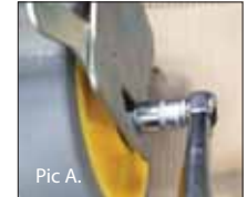
M12 nyloc nut torque to 80Nm. M12 standard washer. Special thin spacer washer on top of swivel bearing of castor M12X60 10.9 bolt
