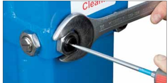
Mast wear screw adjustment
