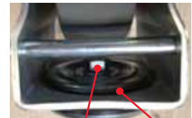
Castor mounting bolt Swivel bearing head should feel free to rotate and not loose
