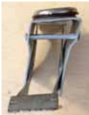
Side impact and foot pedal distortion as a result of a significant side impact.
