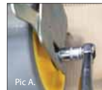
M12 nyloc nut torque to 80Nm. M12 standard washer. Special thin spacer washer on top of swivel bearing of castor. M12X60 10.9 bolt.
